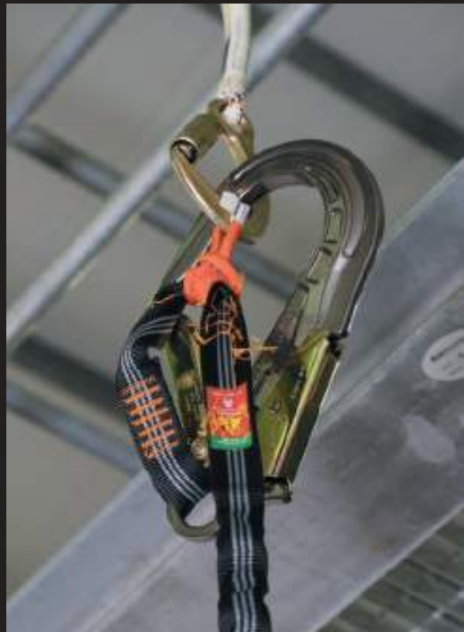
Carabiner of the lanyard can be released.
