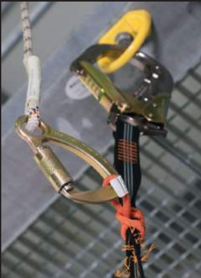
Rescue loop become visible when shock absorber is activated.
